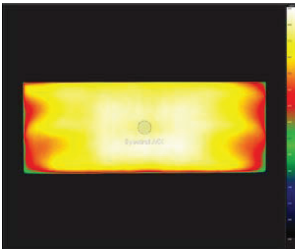
Photometrica software windows showing an example of the display surface pseudo color mapped to luminance, and spectral data in log scale from the measurement spot for white, red, green and blue display settings.
